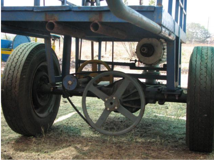
Gear box and pulleys fixed at the end back of a bullock cart. Photo: special Arrangement
