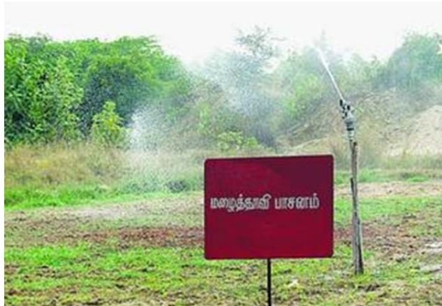
BETTER REACH: A rain gun installed at Agricultural Engineering College and Research Institute at Kumulur. PHOTO: R.M. RAJARATHINAM
