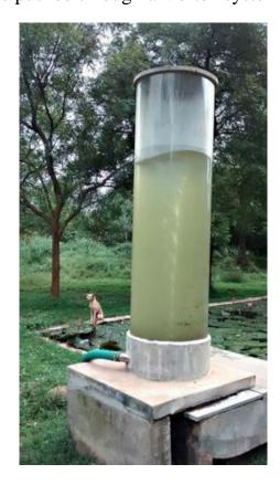
Treated waste-water can be pushed through a Vortex system to reduce odour
