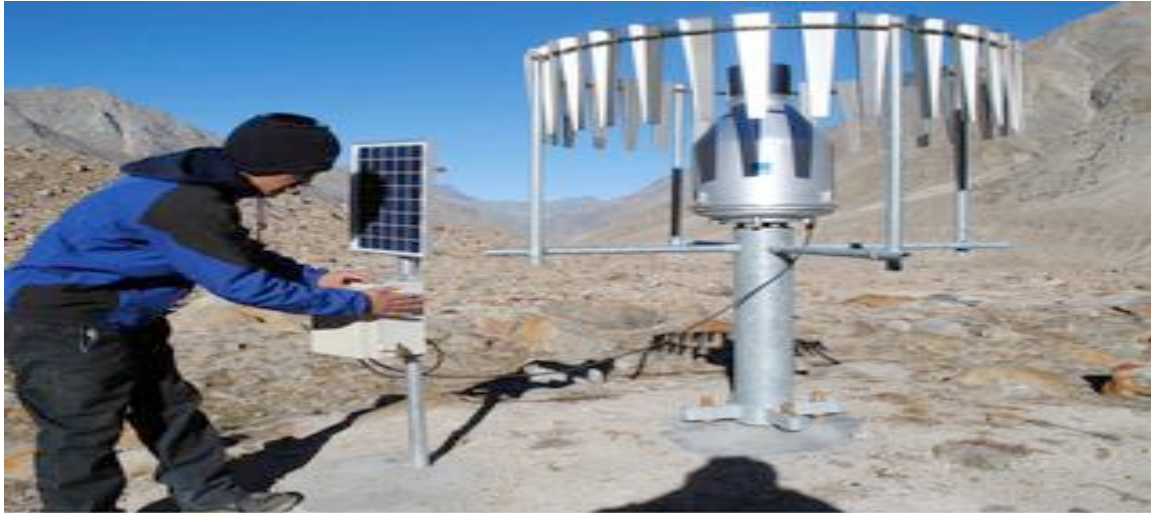
Mohd Soheb checking the precipitation gauge at the JNU base camp. Photo: Special Arrangement
