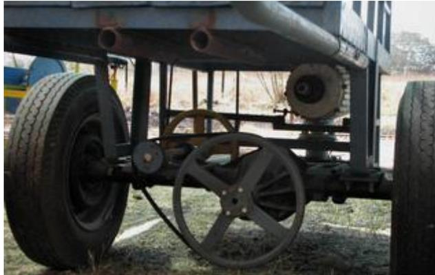
Non conventional: Gear box and pulleys fixed at the end back of a bullock cart.- Photo: special Arrangement
