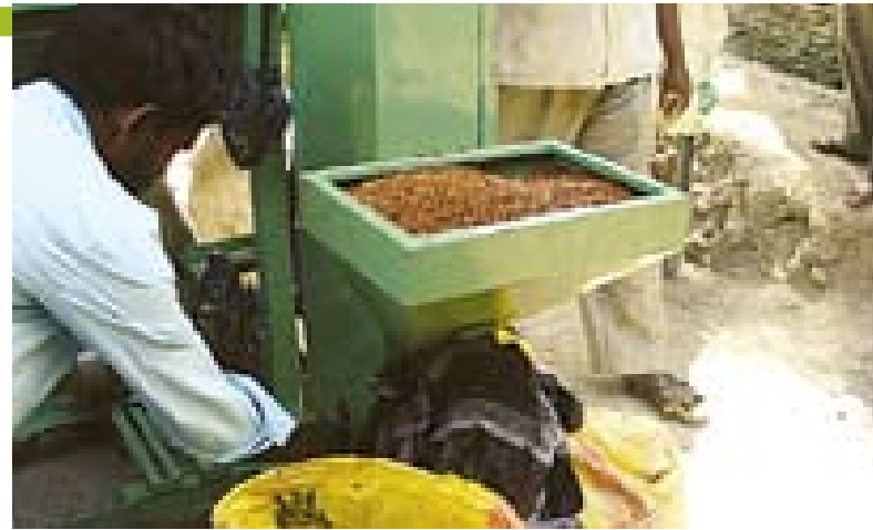
» After Grading Put Tur in Second Machinery (Double Roller Dal Mill )
