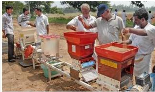
INNOVATIVE IDEA:A new mechanical paddy seedling machine on demonstration at Agricultural Engineering College and Research Institute of the Tamil Nadu
