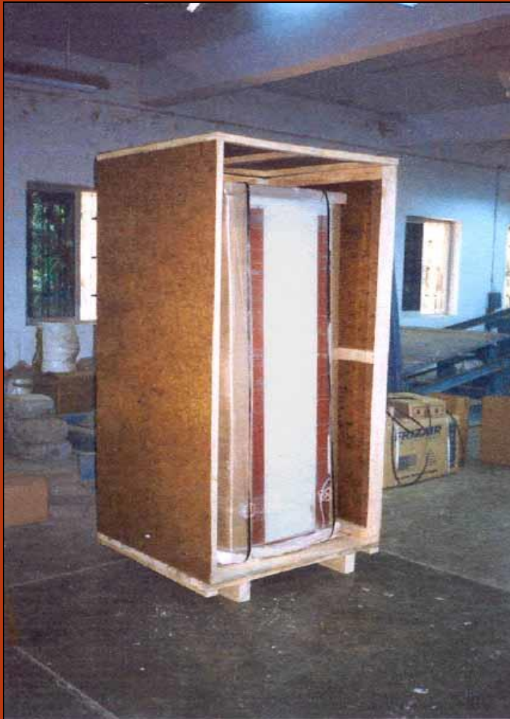
Circuit breaker secured inside Coir Composite Board sheathed Crate.
