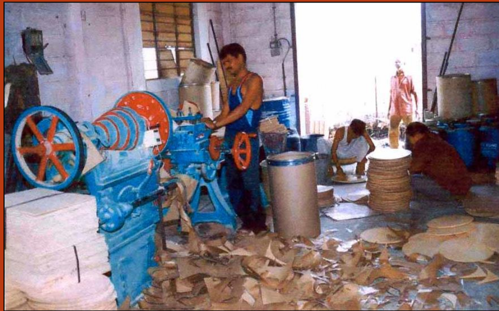
Circular cutting of lids for fibre drums
