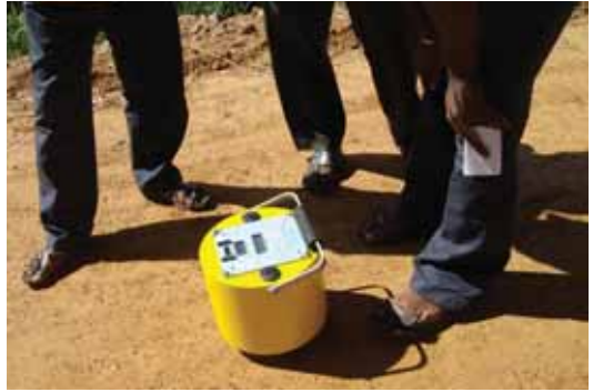
Stiffness & modulus of elasticity determination using Geogauge
