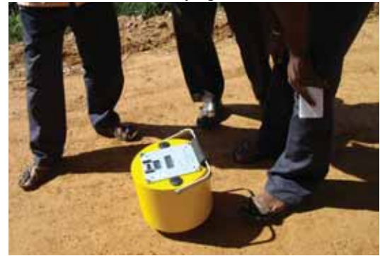
Stiffness & Modulus of Elasticity Determination using Geogauge
