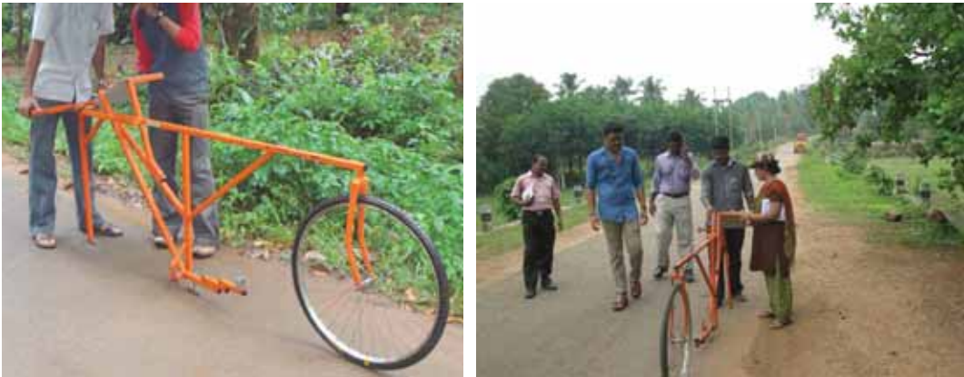
Fig. Merlin test in progress
