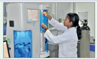
surface area, pore volume and pore size distribution of powdered and porous nano materials. It has a compact, bench-top design with built-in degas capabilities with wide variety of sample cells to accommodate any sample. It can perform automatic analysis including real time display of isotherm data and BET computations and Perform instrument operations locally (via touch-screen) or remotely (via Ethernet-linked PC). It is highly useful for the scientists and students of the University.
