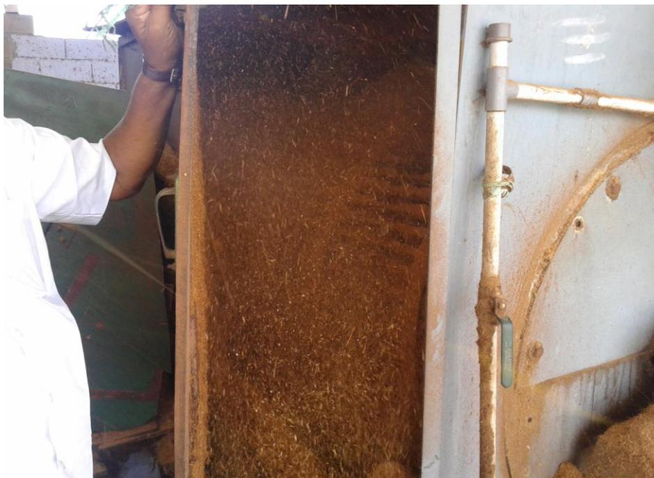
First Quality Fibre is collected seperately and the rest of the contents are sent for further processing
