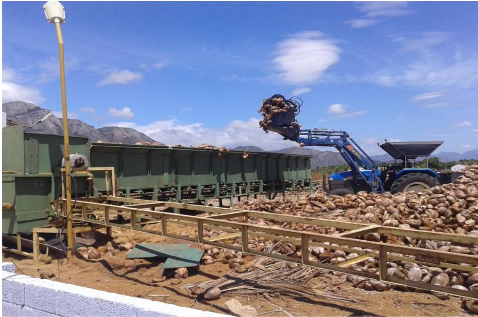
A labour regulates the flow of husk from the hopper on to the moving conveyor
