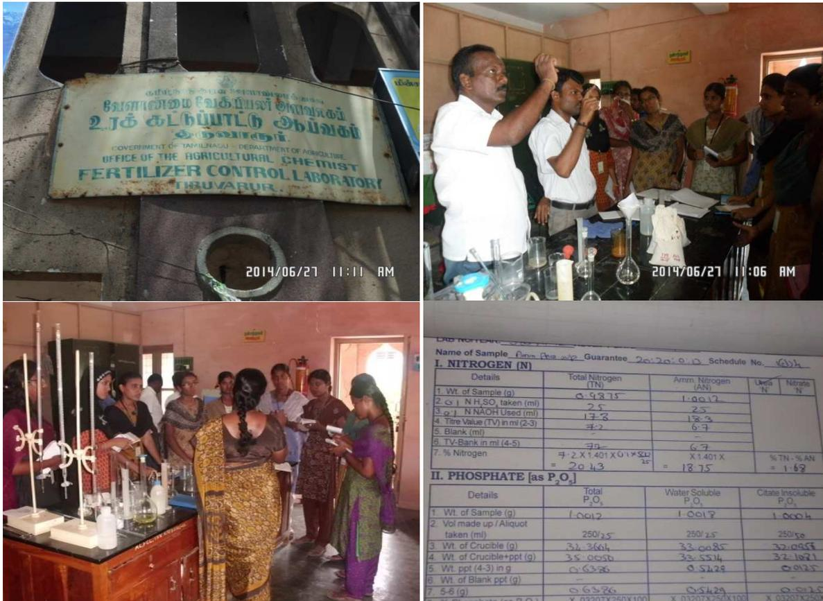
We learned about the objectives and mandates of Fertilizer Control Lab. We had a knowledge on procedures for testing nutrient composition in inorganic fertilizer, period for analyzing the sample, giving result for the particular sample analysis and different forms such as K,L,P form etc., These informations are given to us by Mrs. Arulrani(A.O) .
