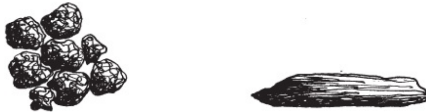
Figure 5.19 Soil is well aggregated by action of colloids rich in calcium ions (left). Soil runs together in a dense mass by action of colloids containing abundant sodium ions (right).
