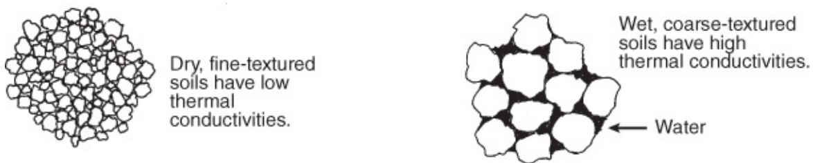
Figure 7.1 The thermal conductivity of a soil depends on its porosity and wetness.
