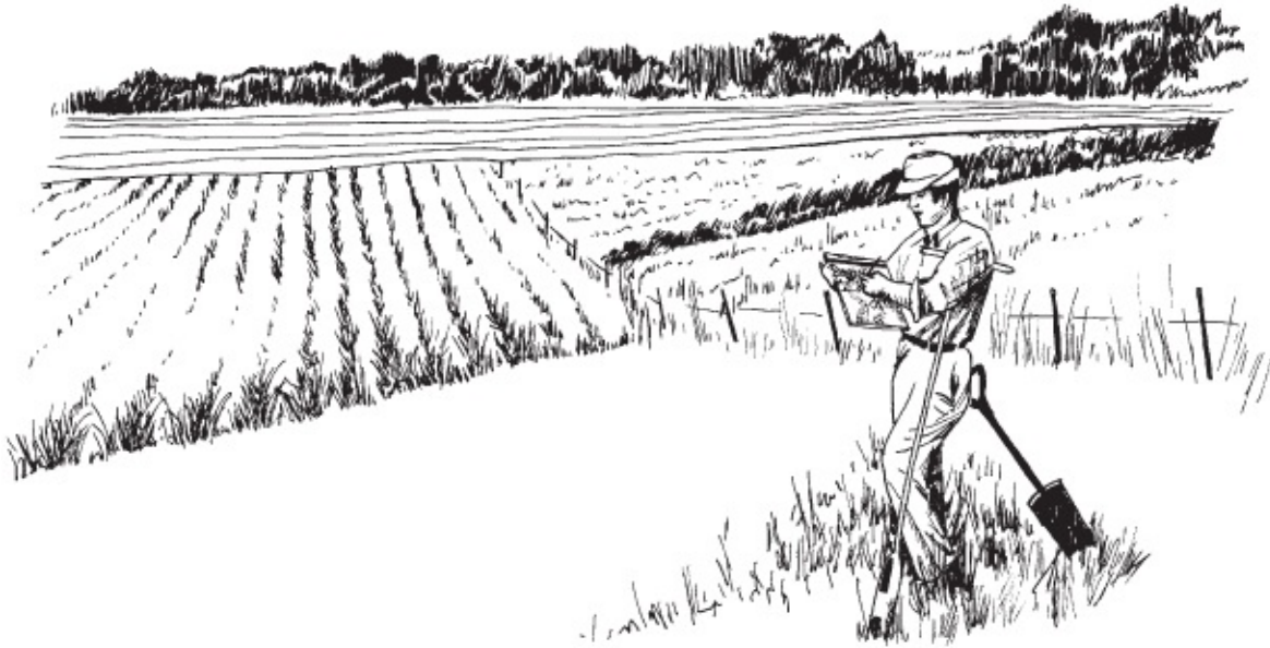
Figure 12.27 A soil mapper makes auger holes to investigate the soil and records the findings on an aerial photograph
