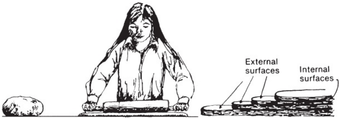
Figure 3.3 A layered clay crystal is similar in nature to a stack of thin sheets of dough.
