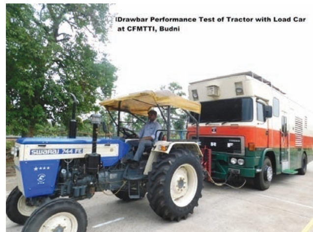
Draw bar testing of tractor at CFMTTI, Budni
