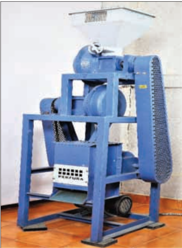
Double stage centrifugal dehuller
